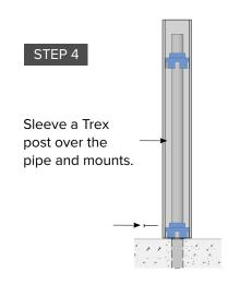
Fasten (1) 3" x #14 self-tapping screw through the Trex post into the bottom donut and pipe.
