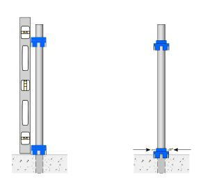
After attaching the top post donuts, use a level to position the lower donuts and attach them to the post using (3) 1" screws.
